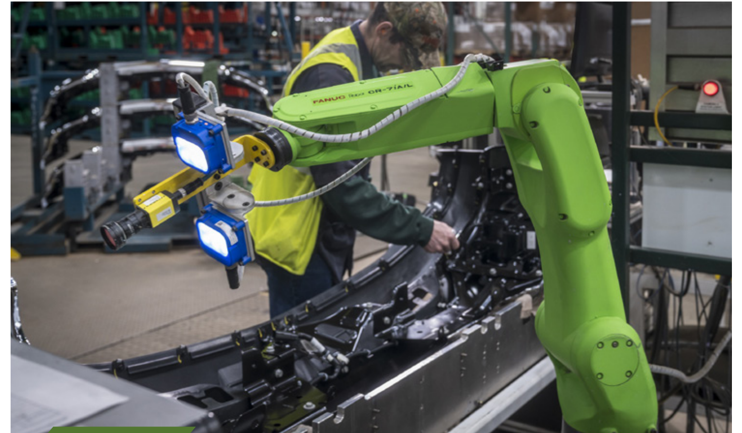
A Fanuc CR-7iA/L cobot equipped with machine vision technology inspects car bumpers for defects working alongside an operator.
